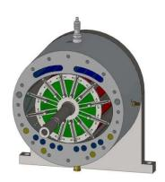
The Circle Ellipse Engine is shown with a transparent End Plate. Unlike the Wankel engine, which implements complex geometry called an Epitrochoid to implement the Otto Cycle, the Circle Ellipse Engine satisfies all requirements of the Otto Cycle with simple, symmetrical geometry.
